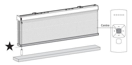
B Deactivate program mode Shortly press the program button to deactivate program mode. The blind stops stepping and can be operated.
