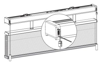
Pair the bottom rail motor to an empty channel on the remote. (see step 1)
